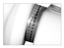
The head is equipped with a goniometer for greater precision during positioning.
