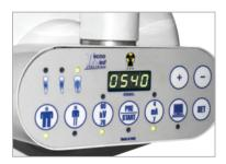
The control panel is located on the monobloc X-ray head for maximum practicality. The default functions can be modified to provide a practical and rapid selection of exposure values for all anatomic conditions and patient requirements.
